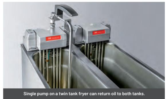
Single pump on a twin tank fryer can return oil to both tanks.
